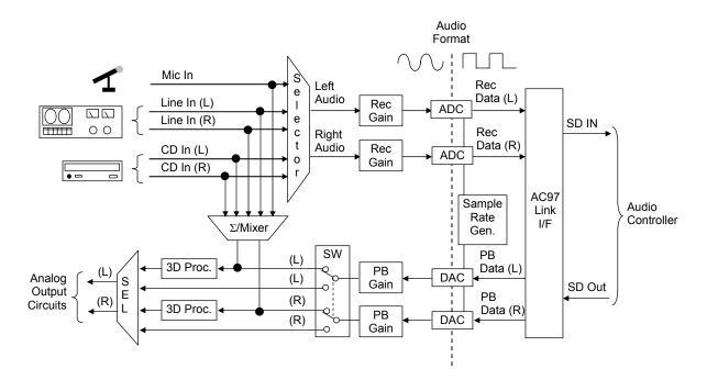
Figure 5-12. AD1885 Audio Codec Functional Block Diagram
